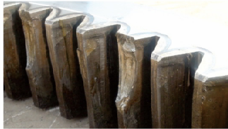
Figure 4 Title: Failure of gear with 37 degree chamfer
