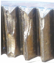
Figure 4 Title: Failure of gear with 37 degree chamfer
